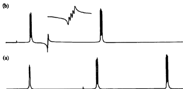
Fig. 1.19. ^1\text{H} spectra of furoic acid- \text{d}_1 , 1.1. (a) Acquired with the spectral width and reference frequency set correctly; (b) acquired with the reference incorrectly set. The inset shows the 'folded' multiplet.
