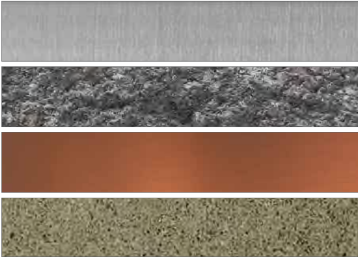
Fig. 8.1 | PROPOSED PRIMARY MATERIAL PALETTE (top to bottom: Zinc, Split-face Concrete Block, Copper, Pre-cast Concrete)
