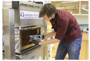
scientists to test instruments to ensure they work in extreme cold before they are sent into space. Before the new CTF was installed, the U of L was capable of testing only smaller instruments in its fleet of cylindrical cryostats. Typically, individual components are tested in laboratories around the world before being integrated in a major space agency facility.
