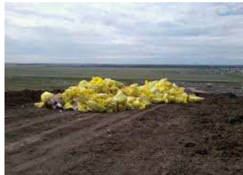
Improperly disposed of asbestos waste
