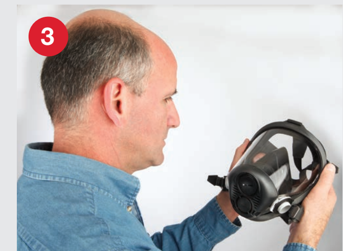
3 Check the lens to make sure it is not cracked or shows signs of crazing.
