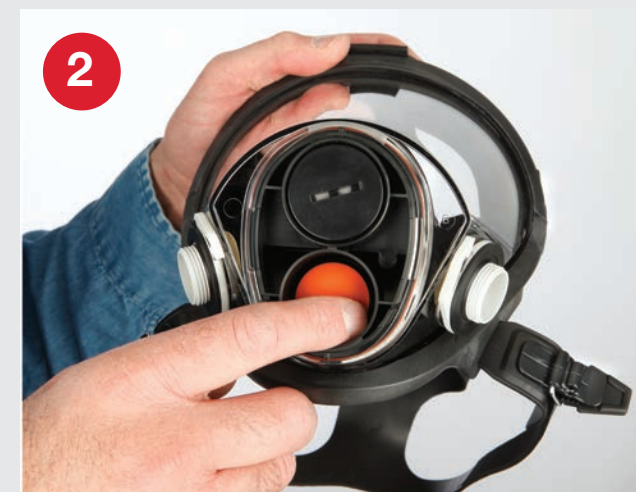
2 Check all the valves to be sure they are present and in good condition. They should be lying flat, without any distortion, tears or holes.
