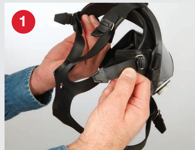
1 Check the facepiece seal & headstraps (or headnet suspension) to make sure they are in good condition, without any holes or tears. Check the cartridge connectors to make sure they are not cracked and are fully inserted into the mask.
