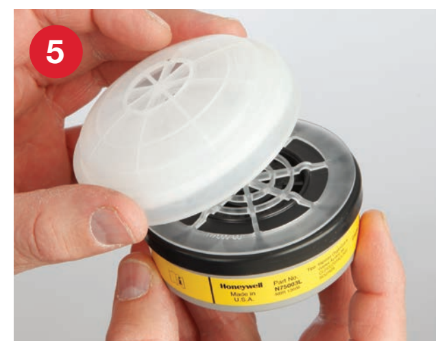
5 Place the pad filter support on top of the cartridge, "groove side up". Then, snap the filter cover onto the cartridge or N750037 filter holder and cover (if a cartridge is not being used).
