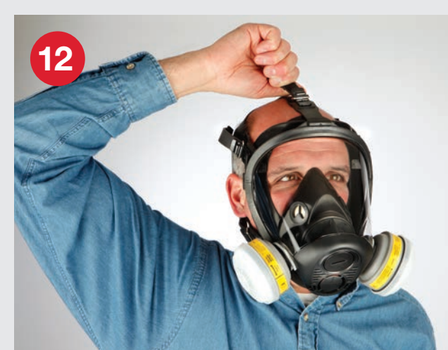
12 If you have the 7600 five strap harness, tighten the forehead headstrap. The facepiece should be snug, comfortable and centered on your face. DO NOT OVERTIGHTEN any of the suspensions.
