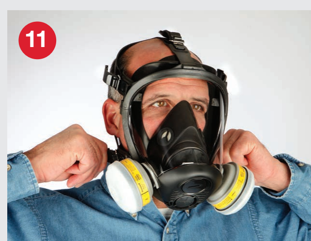
11 For all three suspension types (5-strap, 4-strap, and headnet), start with the lower straps, tighten both sides evenly. Or, with one hand holding the front of the facepiece, use your free hand to tighten each strap alternately in small, equal increments. Then, tighten the upper straps on either side of the forehead. If you are using the RU6500 with headnet, smooth the headnet over the top and back of your head until lying flat.
