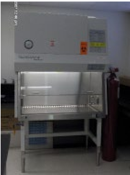
Figure E-1: Biological safety cabinet. The picture shows an example of a class II-A cabinet, which does not have a hard-ducted exhaust system. The front sash has an optimal height setting to minimize disruption of the protective air curtain at the front of the work area. Moving the sash higher than this optimum setting will cause the cabinet to alarm.
