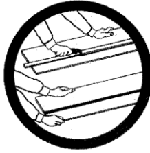
Cutting asbestos-containing wall board by hand
