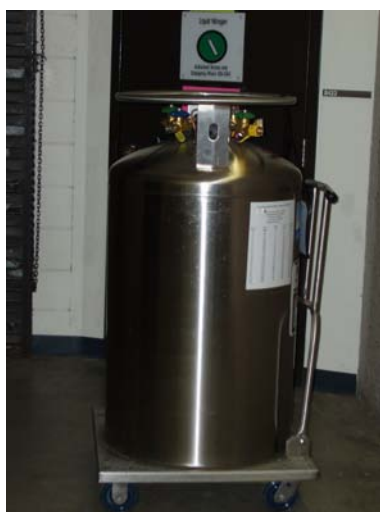
Figure 2. Pressurized Dewar flask (left); valve system (right).
