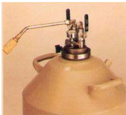
Figure 3. Dewar and transfer tube.
