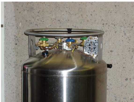
Figure 2. Pressurized Dewar flask (left); valve system (right).
