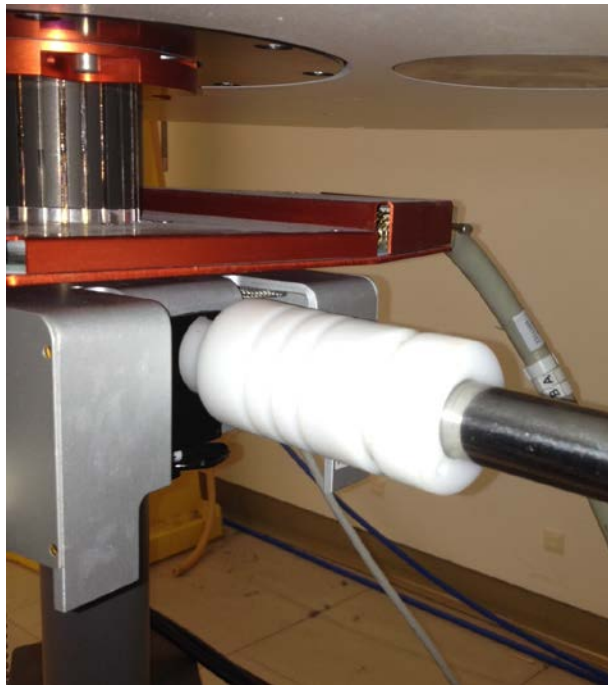
Figure 8 Picture of the LN2 VT line attached to the probe.
