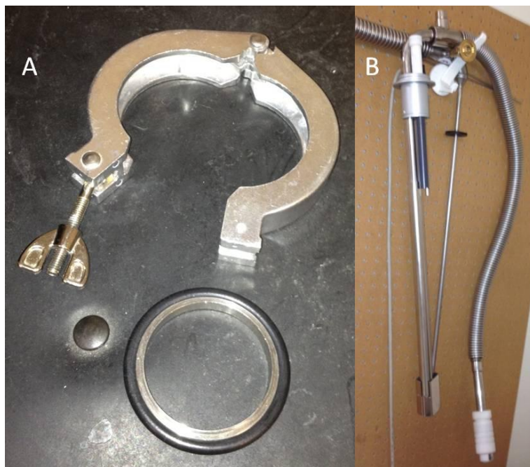
Figure 4 (A) O-ring and ring clamp (B) VT Line for LN2 use
