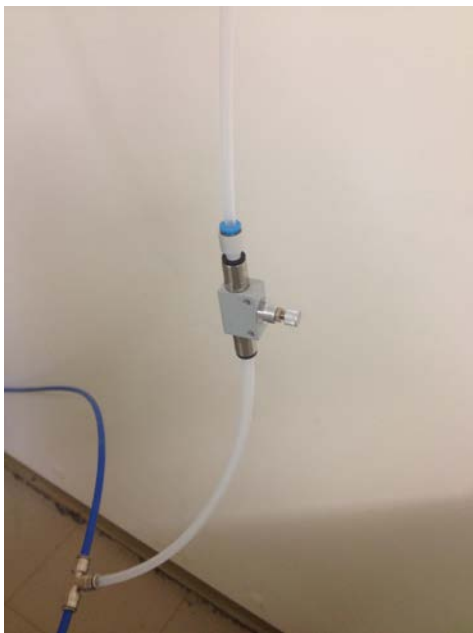
Figure 1: Valve for air flow through the shim supply
