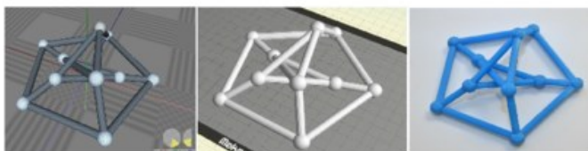
The Petersen graph, as it appears in GLuskap, MakerBot® Makerware, and as a printed model.
