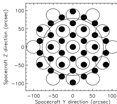
Figure 1. The layout of the SPIRE iFTS detector arrays. SSW pixels are shown as filled circles and SLW as empty circles. The 2.6' unvignetted field of view is also shown.
