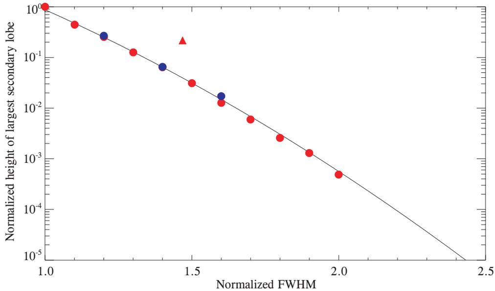
Fig. 2. Filler diagram of the 10 apodizing functions described in this paper (red circles) and the three original ones of Norton and Beer (blue circles). Also shown is the locus of the commonly used triangle apodizing function (triangle).
