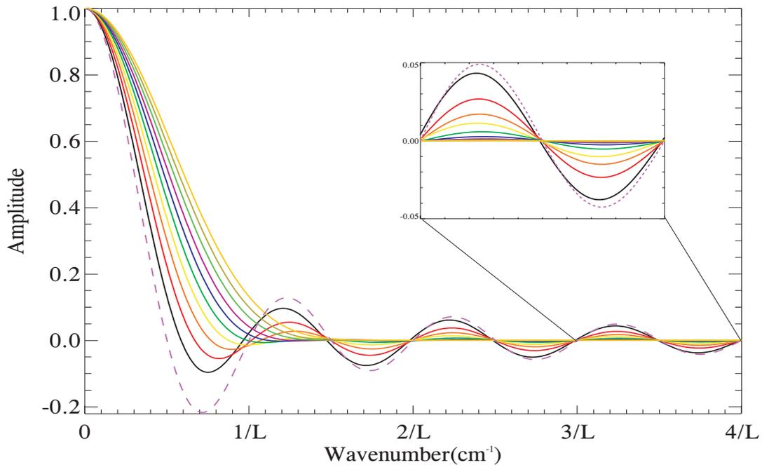
Fig. 1. Instrumental line shapes corresponding to the 10 apodizing functions described in the text compared with the sinc function (dashed line). Inset shows the magnified region of the third sidelobe.
