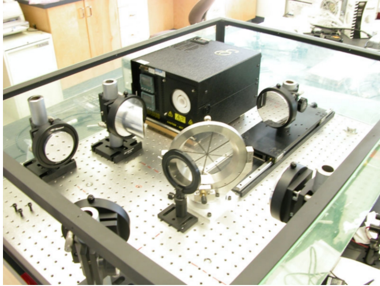
Figure 6.1: A picture of the TFTS during verification testing. The beamsplitter shown is used for optical alignment. A diagram of the TFTS with components labeled is shown in figure 6.2. The image is courtesy of the AIG.
