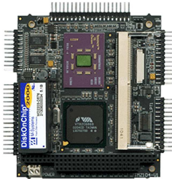
Figure 5.3: Tri-M TMZ104 PC/104 single board computer, powered by a 667 MHz Transmeta Crusoe 5500 CPU.
