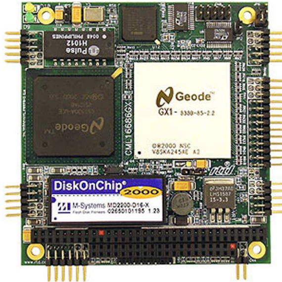
Figure 5.4: RTD CML16686GX333HR PC/104 single board computer, featuring an on-board Ethernet controller. The computer is powered by a 333 MHz National Semiconductor Geode CPU.
