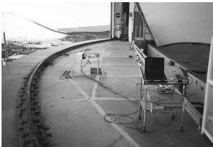
Figure 5: The infrared radiometer, electronics package and laptop control computer on the apron of the JCMT.
