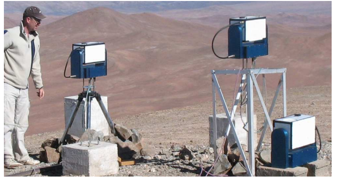
Fig. 1. Greg Tompkins with the three TMT IRMA units during the calibration verification on site.
