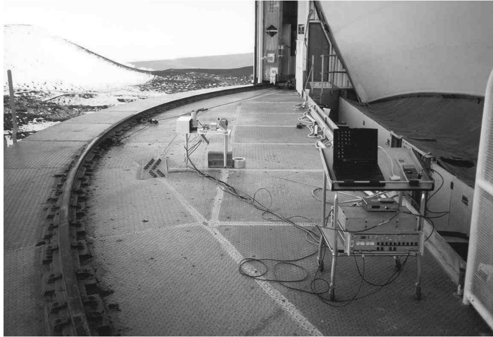
Figure 4.1: A view of the prototype radiometer showing the instrument platform at the center of the skirt of the JCMT and the instrumentation located some distance away.
