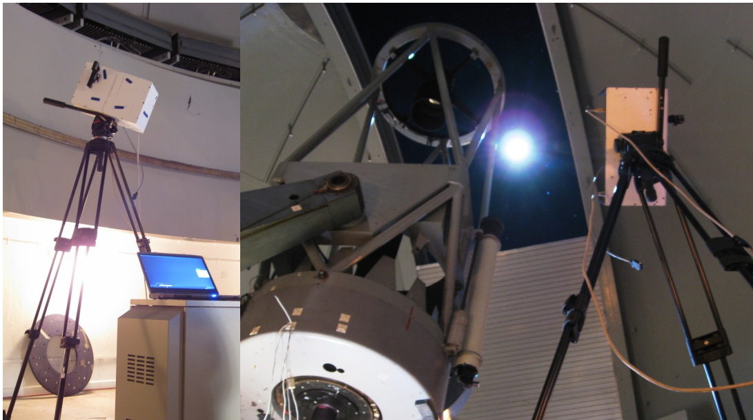
Figure 6. The lunar spectrophotometer mounted on a tripod (left). The moon, as viewed through the open dome above the ESO, 1-meter telescope at La Silla Paranal Observatory, Chile (right).
