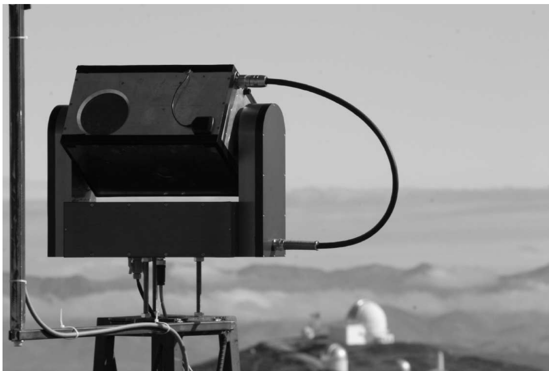
FIG. 1.—IRMA radiometer and altitude-azimuth mount stationed at the Las Campanas Observatory, Chile.
